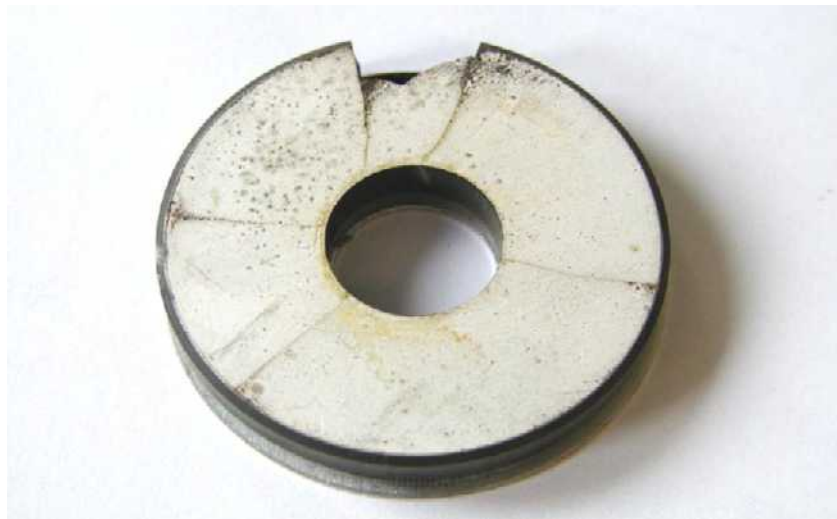
Illustration 14.1. Torn and broken piezoceramics
