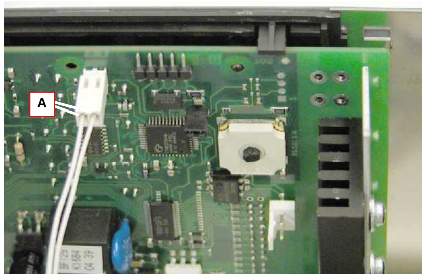
Illustration 5.3. Measuring points PCB control
