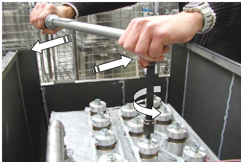
Illustration 14.2. Always hold the torque wrench vertically. Do not tilt the tool!
