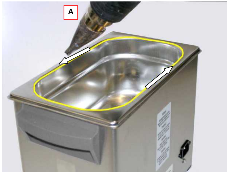
Illustration 15.3. Heat up the edge of the transducer tank with a hot air fan
